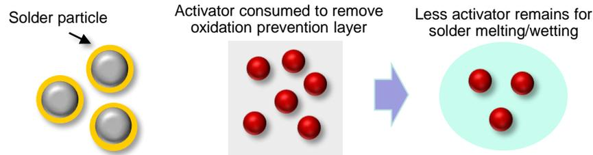
Considerable activator is consumed to remove the thick oxidation prevention layer. Subsequently limited activator remains for wetting/melting.
