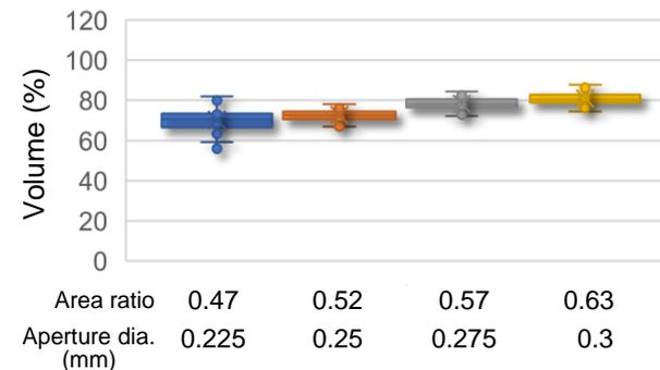
➤ Consistent paste transfer volume from the initial paste print even after 60 min. pause even with area ratio  $\geq 0.52$ .
