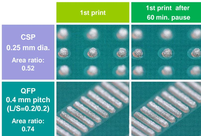
$$\text{Area ratio} = \frac{\text{Aperture area}}{\text{Aperture wall area}}$$
