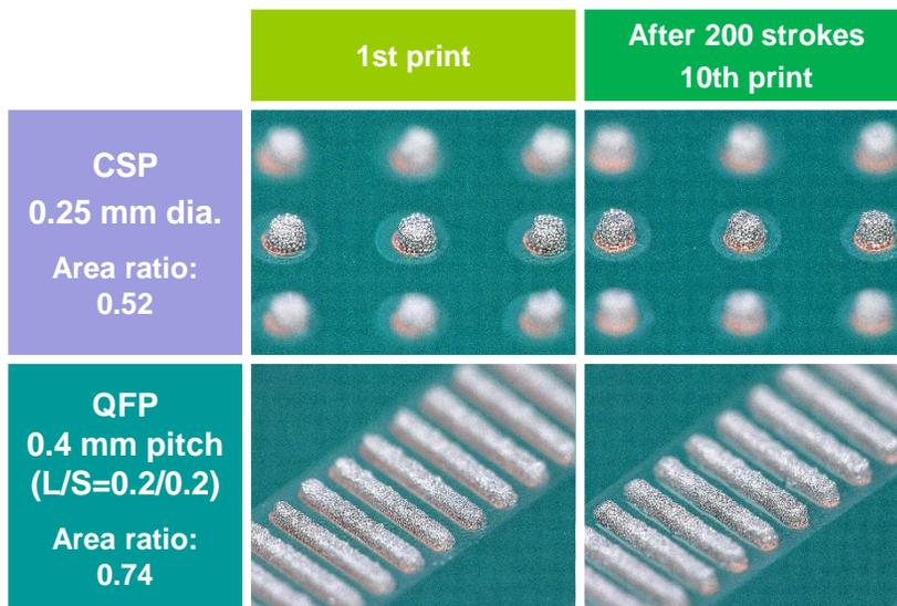
$$\text{Area ratio} = \frac{\text{Aperture area}}{\text{Aperture wall area}}$$
