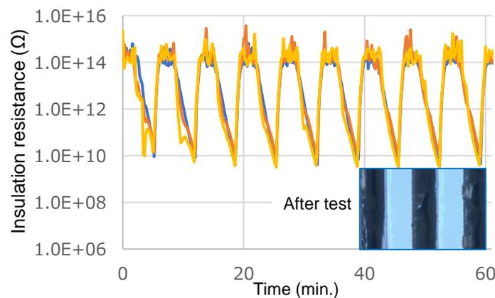
➤ **S3X58-HF1100-3** showed robust high reliability under harsh conditions, with no evidence of dendrite growth observed.
