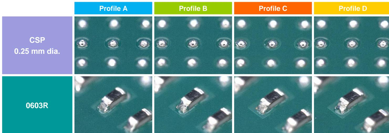
➤ S3X58-HF1100-3 shows good meltability without dependency on the type of reflow profile used.
