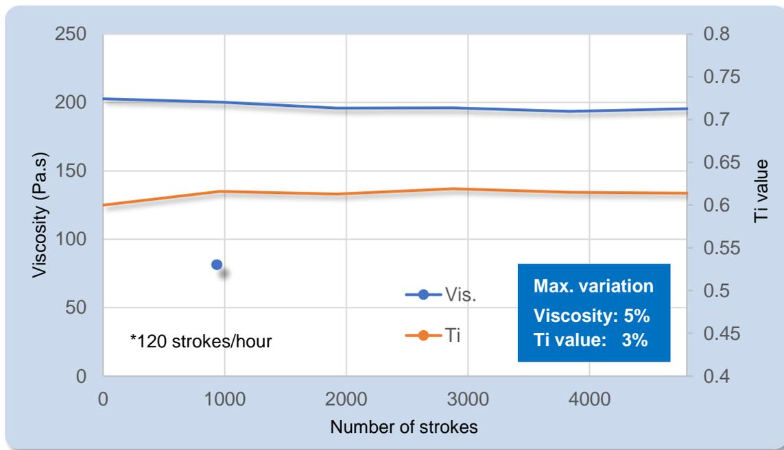
➤ Continual paste print strokes with periodical paste replenishment resulted in stable rheology (viscosity and thixotropy).
