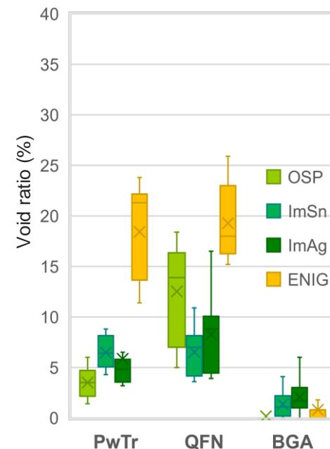
➤ Consistently low voiding is achieved with each type of component and surface finish.
