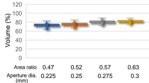
➤ Consistent print quality with good printed paste shape even with area ratio  $\geq 0.52$ .
