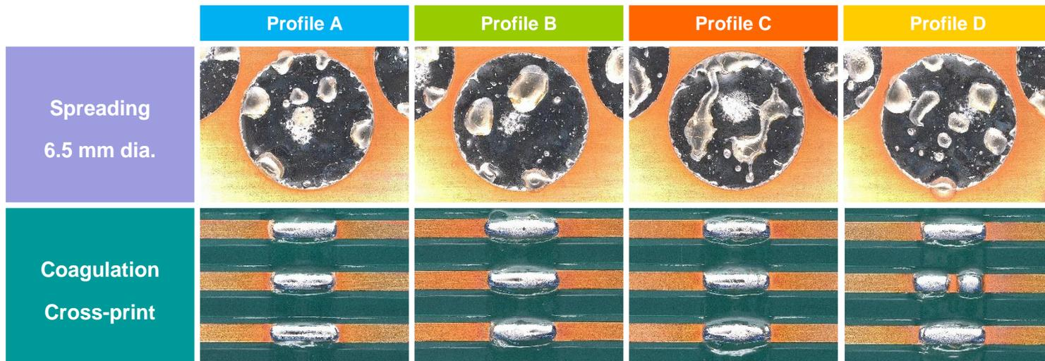
➤ **S3X58-HF1100-3** resulted in good spreading and no solder balls were left in-between tracks after coagulation without dependency on the type of reflow profile used.
