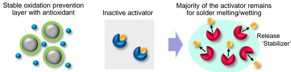
Solder particles are protected from being oxidized by an easy-to-remove protective layer and the antioxidant suppresses continued oxidation over time. Such effects help save the amount of activator needed for oxidation prevention, as well as the activator capping technique which allows maximum activation strength when the solder is molten.
