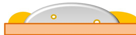
**Coagulated liquefied flux effectively and swiftly evacuates** out of the solder joint and leaves significantly low voids.
