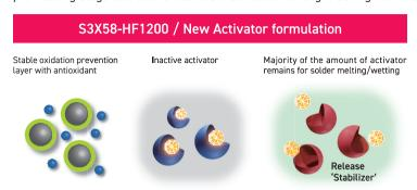
Solder particles are protected from oxidation by a removable layer, and antioxidants further prevent it over time. This reduces the activator needed and enhances activation strength when the solder is molten.
